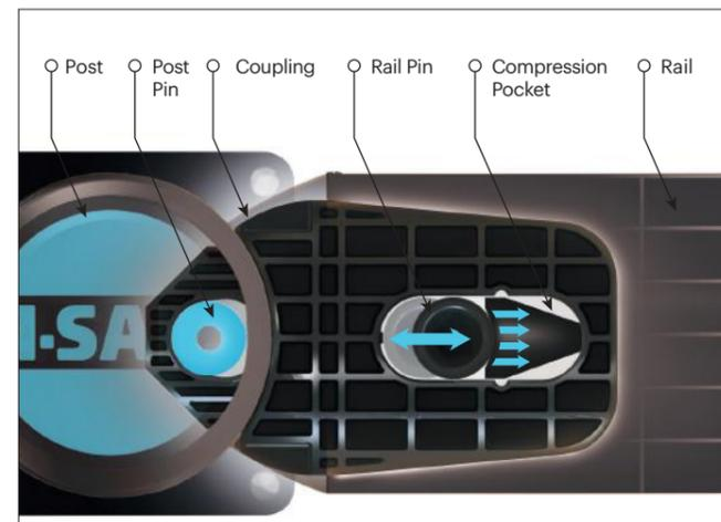
**PHASE 1:** Memaplex™ rail flexes to absorb impact, initiating the rail pin to slide forward and transfer load energy to the compression pocket.
