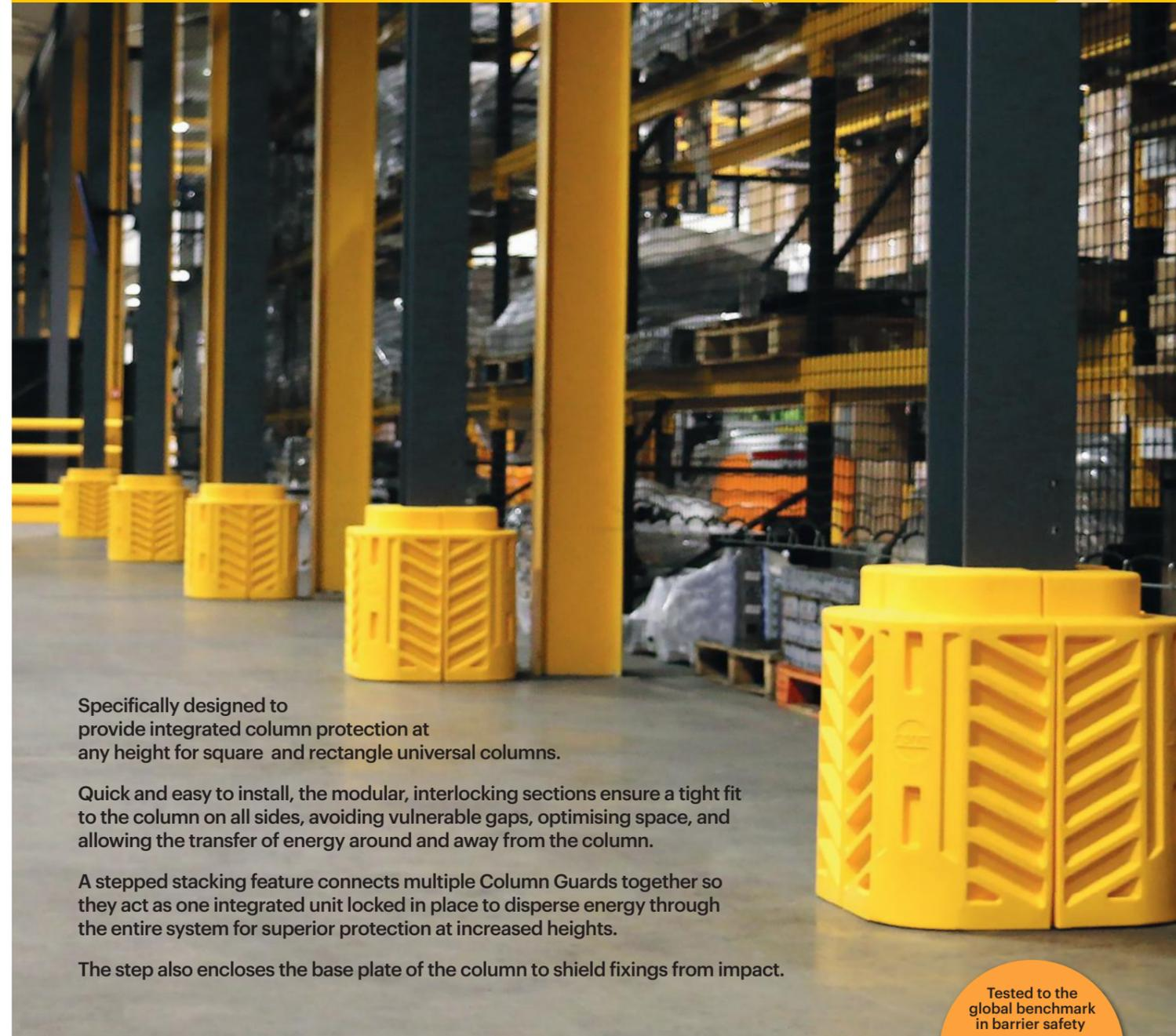
Specifically designed to provide integrated column protection at any height for square and rectangle universal columns.
